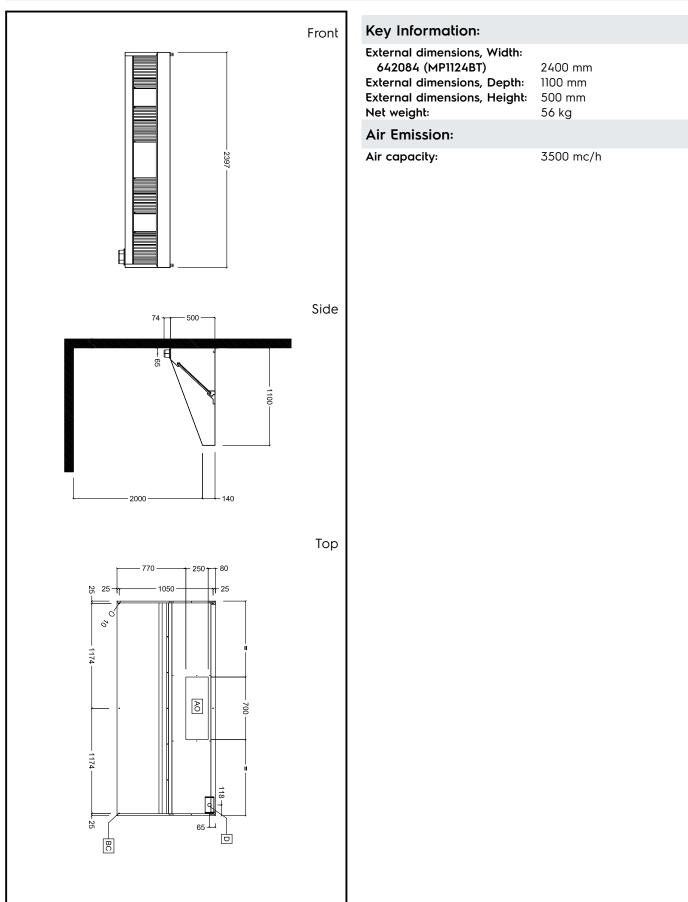
Ventilation Equipment 430 S/S Wall Hood+Filters 2400X1100mm
